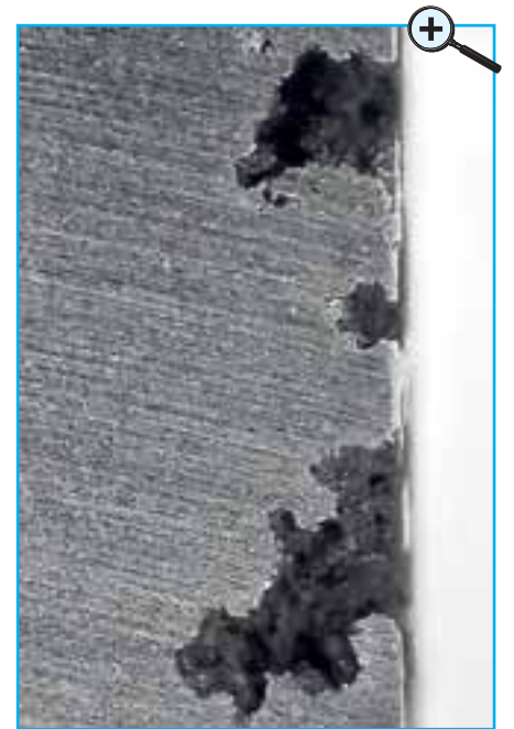
Fig. 3 cross section of liner
